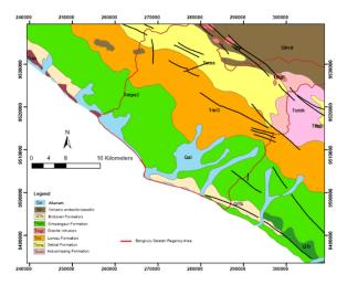
Figure 2. Geology map of Bengkulu Basin (Amin et al., 1993; Setyowati et al., 2018)
