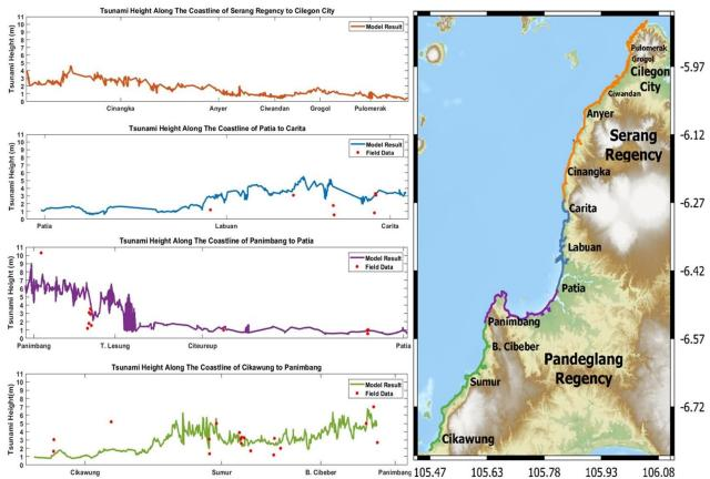
Figure 4. Maximum tsunami elevation along the Pandeglang Regency to Cilegon City and overlaid with tsunami height from a field survey conducted by Indonesian Geological Agency (the red dots). The orange line shows the coastline along Cinangka-Pulomerak sub-district, the blue line shows the coastline along Patia-Carita sub-district, the purple line shows coastline along Panimbang-Patia sub-district, the green line shows the coastline along Cikawung-Panimbang sub-district.
