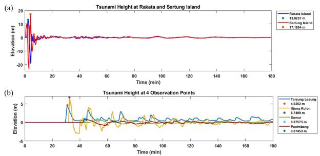
**Figure 6**. Tsunami height from simulation are shown at: (a) observation point 42 (Rakata Island), and observation point 43 (Sertung Island), (b) observation point 44 (Tanjung Lesung), observation point 45 (Ujung Kulon), observation point 48 (Ujungjaya, Sumur), and observation point 49 (Panimbangjaya, Panimbang).
