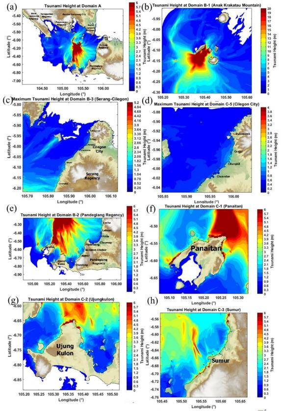
Figure 7. Tsunami height map from the simulation at: (a) Domain A, (b) Domain B-1 (Anak Krakatau Volvano), (c) Domain B-3 (Serang Regency to Cilegon City), (d) Domain C-5 (Cilegon City), (e) Domain B-2 (Pandeglang Regency), (f) Domain C-1 (Panaitan Island), (g) Domain C-2 (Ujungkulon), (h) Domain C-3 (Sumur), (i) Domain C-4 (Panimbang-Labuan), (j) Domain D-2 (Tanjung Lesung).
