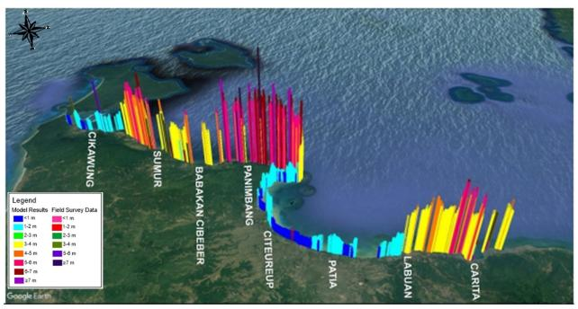
Figure 5.Tsunami height map from the simulation and field survey (Indonesian Geological<br/>Agency) along the Pandeglang coast
